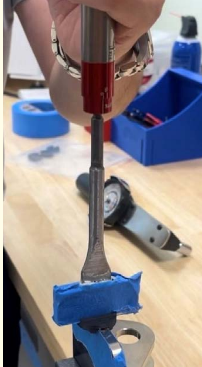
An engineer with the NAVAIR AM team uses a torque wrench to test the part's breakaway requirement.
