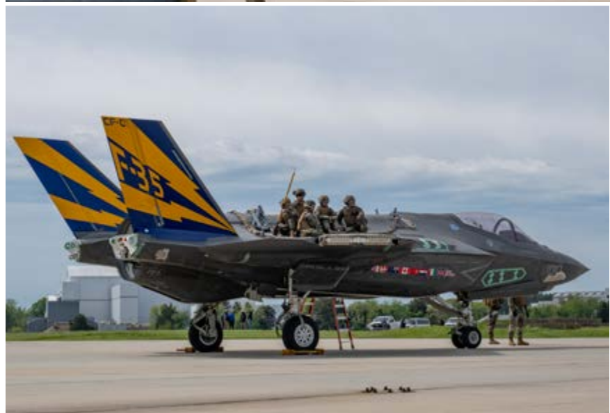
Members of the HST from the Marine Corps Combat Logistics Battalion 26 sit poised atop CF-1, a non-flying F-35C airframe from the NAS Patuxent River F-35 Integrated Test Force, waiting to hook the airframe to sling hoists lowered from a CH-53K being flown by Marines from VMX-1. The airframe, lifted and transported via CH-53K, was flown from NAS Patuxent River, Maryland, to Joint Base McGuire-Dix-Lakehurst, New Jersey, April 24 to support future testing of emergency recovery systems.
