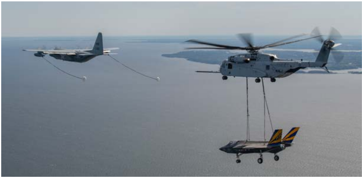
Marines from VMX-1 pilot a CH-53K helicopter over the Chesapeake Bay in Maryland, conducting aerial refueling from a C-130T operated by Navy's VX-20 while carrying a non-flying F-35C test airframe from the NAS Patuxent River F-35 Integrated Test Force on April 23. The flight was conducted in preparation for the aerial transport of the non-flying F-35C airframe from NAS Patuxent River, Maryland, to Joint Base McGuire-Dix-Lakehurst, New Jersey, the following day.
