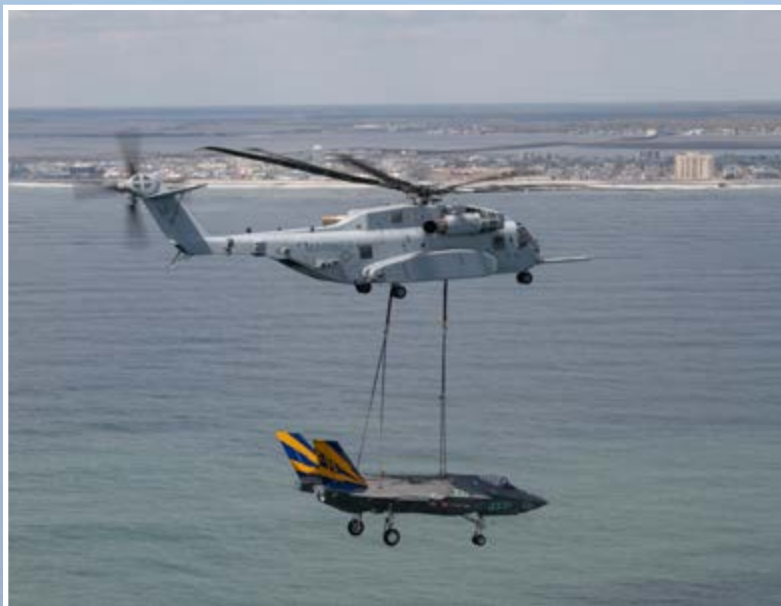
A CH-53K, piloted by Marines from VMX-1, flies along the coast of Ocean City, New Jersey, with a non-flying F-35C test airframe from the NAS Patuxent River F-35 Integrated Test Force carried beneath it April 24 during an aerial transportation of the test aircraft from NAS Patuxent River, Maryland, to Joint Base McGuire-Dix-Lakehurst, New Jersey.
